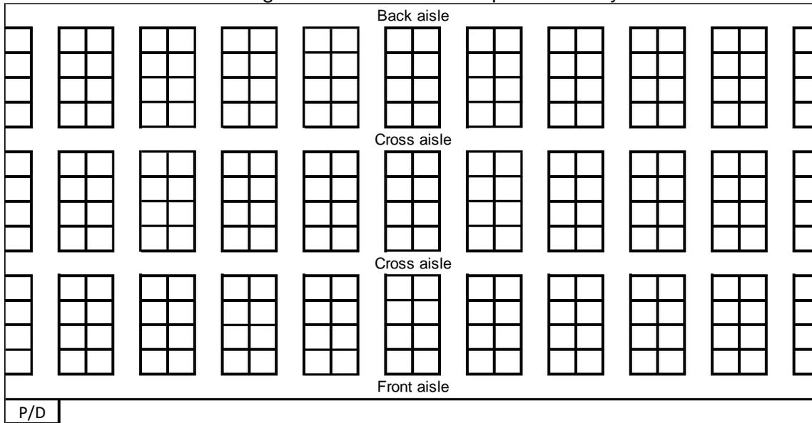
Figure 3: Uneven cross-aisle placement layout
