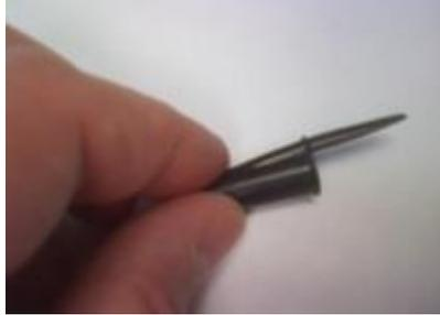
Then I ask the students to compare that to a defective pen cap I acquired as a young boy. The cap is shown in Figure 11. While I am not 100% sure of the cause of the error, it does provide an opportunity to discuss the danger of tools or fixtures that can be aligned either correctly or with a turn of 180%. This pen cap could have been produced with an injection mold where the top was turned 180% from the correct orientation.
