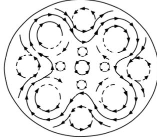
Figure 3. Asymmetric flow observed in Fultz's dishpan experiment
